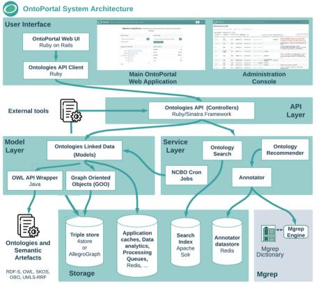
Fig. 2. OntoPortal system architecture.
